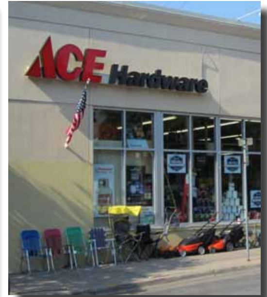
NOT RECOMMENDED Internally lit cabinet box/letters are not an appropriate wall sign type.
